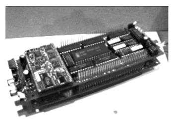
Figure 3: The Cognachrome Color Tracker mounted on the Vesta Processor Board
