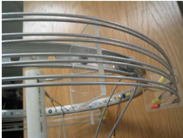
Figure 6: Bar codes , made of steel wool, shorted out certain pairs of rings when the robot ran into them.
