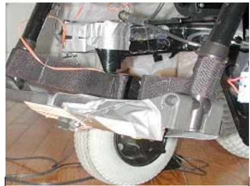
Figure 1: Drop-off Detector mounted on an Invacare Action Arrow (Invacare, Elyria, OH)
