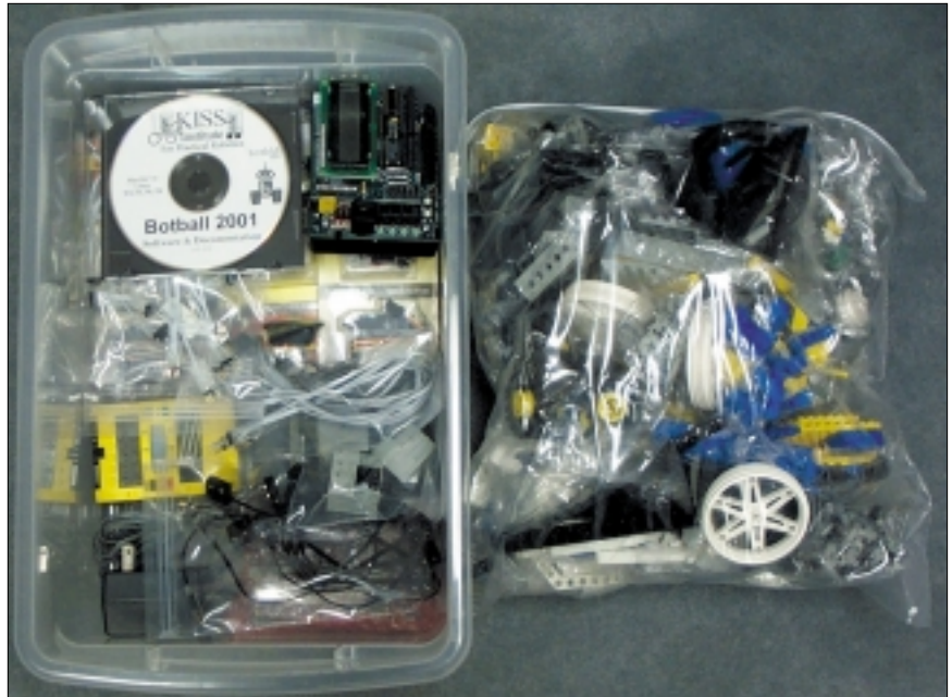
Figure 1. Botball kits include two microprocessors, about 20 sensors, 10 motors, and almost 2,000 LEGO pieces.
