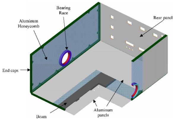
Figure 3: *Chassis Box Cutaway*
