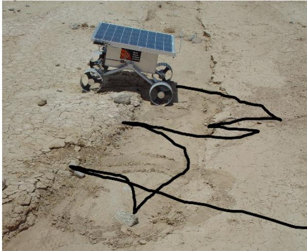
Figure 6: *SR2 moving along a ridge-line until an acceptable slope is found (pathline added)*
