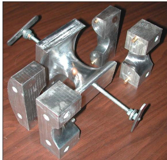
Figure 4: *Inner & outer wheel spoke molds*
