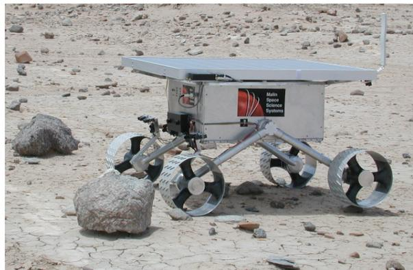
Figure 1: *The SR2 Rover Maneuvering Between Obstacles During a Field Test in the Salton Sea Desert*
