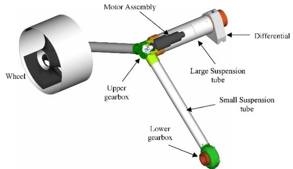
Figure 2: *Drive Train Cutaway*
